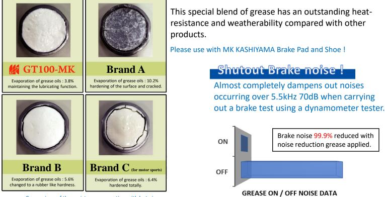
Comparison of the moisture evaporation with hot air circulating in a constant temperature bath of 250°C after 7days.
