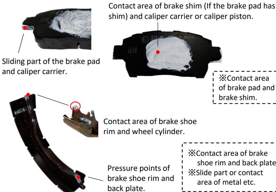
Contact area of brake shim (If the brake pad has shim) and caliper carrier or caliper piston.
